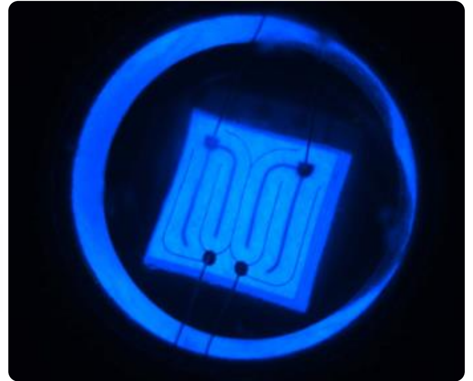
RPCVD 'Active as-grown' (AAG) tunnel junctions are a potential solution to address efficiency droop in high-brightness LED applications
