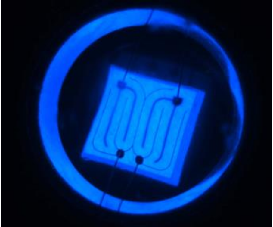
RPCVD 'Active as-grown' (AAG) tunnel junctions are a potential solution to address efficiency droop in high-brightness LED applications
