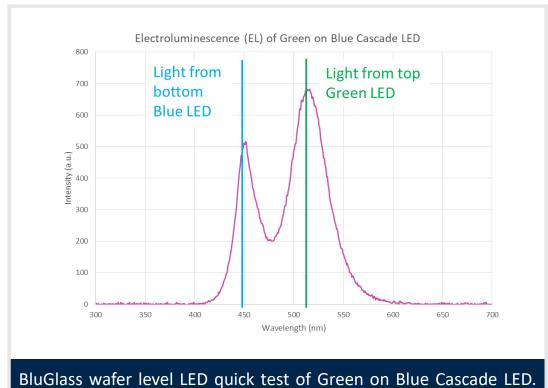
BluGlass wafer level LED quick test of Green on Blue Cascade LED. The emission spectrum shows two peaks, one from the blue active region and one from the green active region – the signature of a cascade LED.
